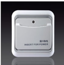
60526-50 Card switch, AC220V±10%, 16AX resistive or 8AX inductive
